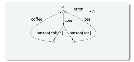
A machine with an error. The occurrence of an error is actually rather an internal action and could alternatively be modelled with a  $\tau$ .
