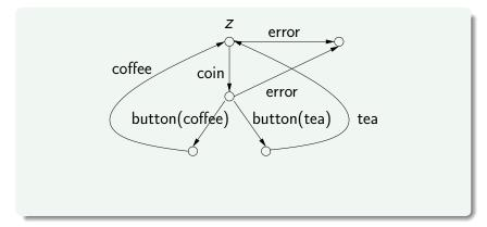
An (unfair) machine with faulty behaviour which may enter the error state after a coin has been inserted.
