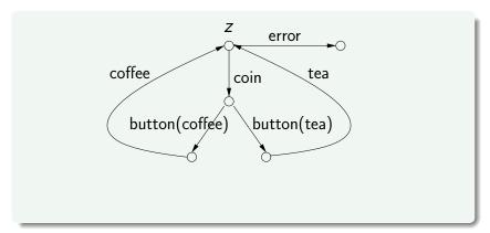
A machine with an error. The occurrence of an error is actually rather an internal action and could alternatively be modelled with a au.
