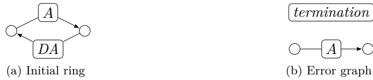
Figure 7.3.: Graphs describing the initial and erroneous configurations of the termination detection protocol
